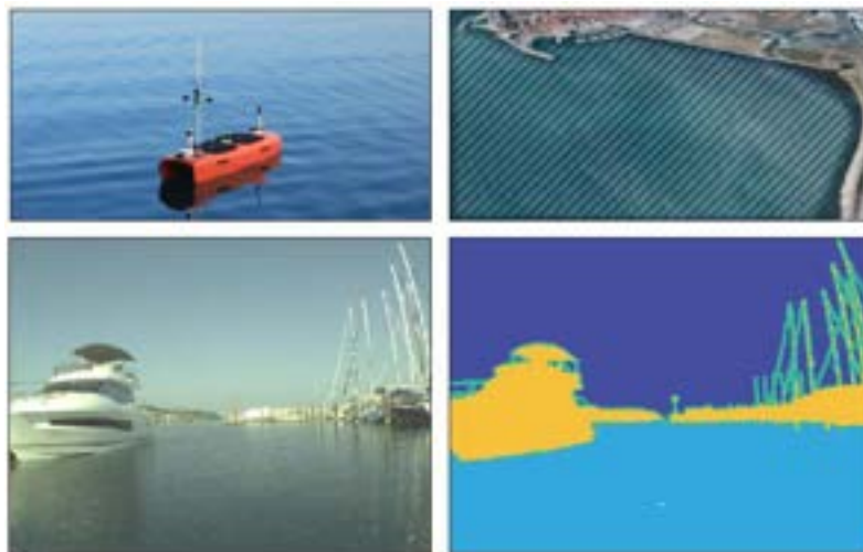
A USV and example of semantic segmentation for obstacle detection.
