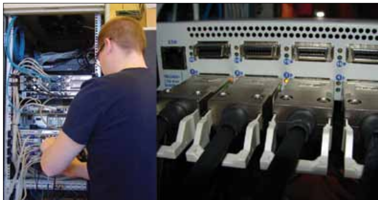
Interconnecting four servers in a cluster via 20 Gbps low latency Infiniband links
