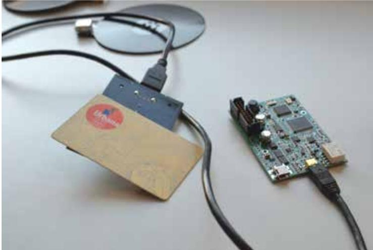
Proxmark system for reading and writing contactless cards.
