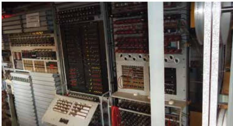
Colossus was the first electronic computer, used by British codebreakers during World War II for cryptanalysis of the Lorenz cipher
